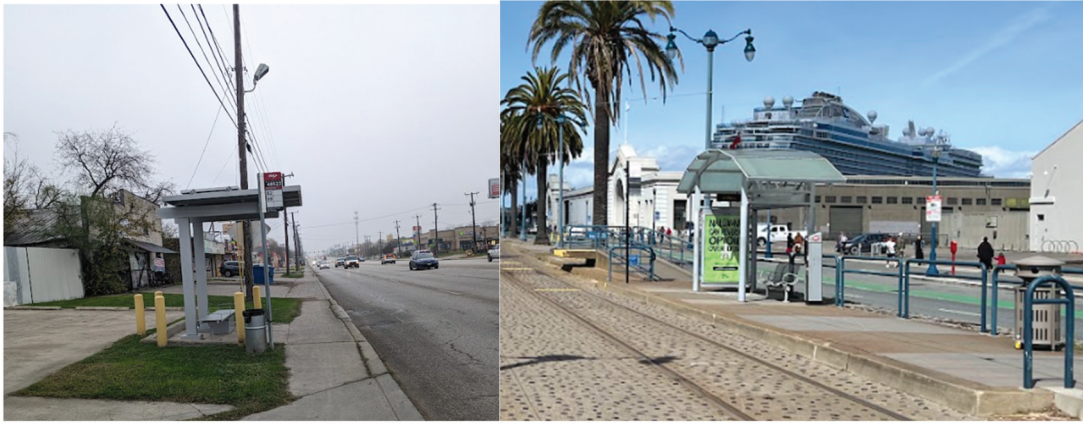
Figure 8. Transit stops with shading, seating, protected shelters setback from the road, and trash service (San Antonio (TX); San Francisco (CA), 2022-2024. Credit: Author).
